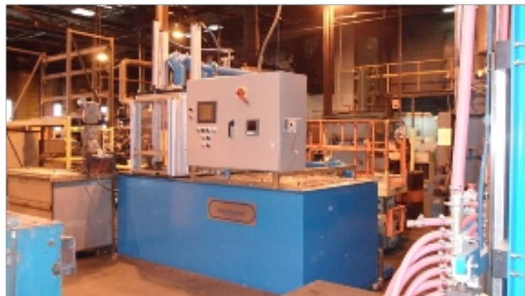
Figure 7 High-velocity IQ system for processing parts of up to 200mm diameter and 500mm length installed at Euclid Heat Treating Co.
