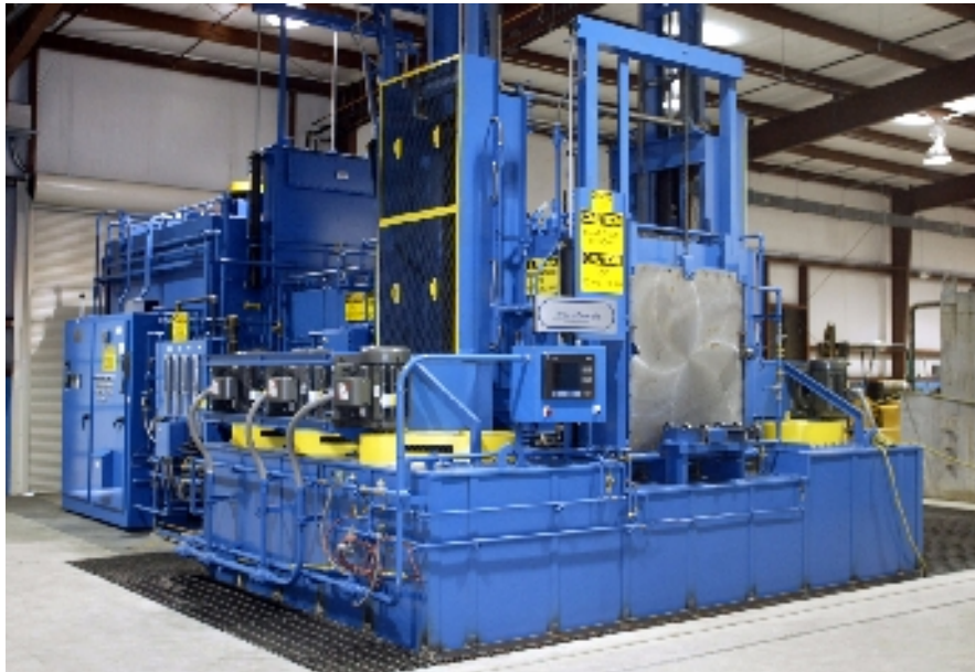
Figure 5 AFC-Holcroft Integral Quenched Furnace Equipped With 11,000-gallon IQ Water Tank and Installed at Euclid Heat Treating Co.
