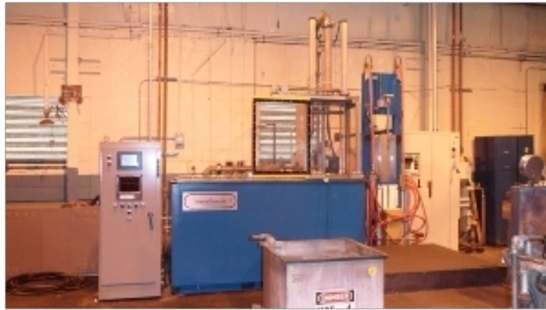
Figure 8 High-velocity IQ system for processing shafts of up to 50mm diameter and 910mm length installed at Euclid Heat Treating Co.
