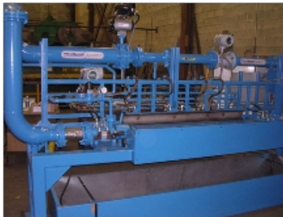
Figure 9 High-velocity IQ system for processing torsion bars
